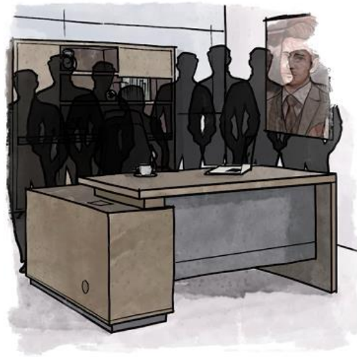
Unrealistic Occupant Load for Single-Person Office [Incorrect] (Maximum Possible Number of Occupants within a Space)
