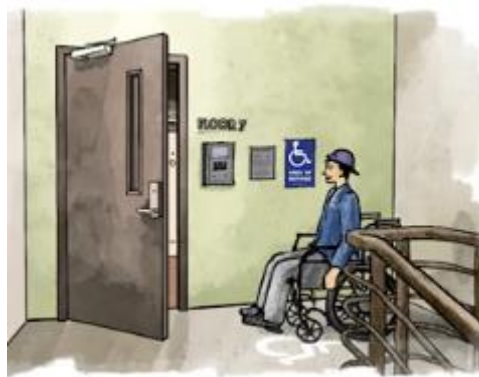
Allow Time to Protect-In Place (Area of Refuge within an interior exit stair)
