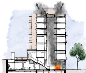
Design of an Engineered Smoke Control System
