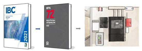
The 2021 IBC determines when a fire alarm system is required, then invokes NFPA 72 (2019 Edition) for how to design and install the system.
