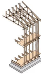
Framing (Structure or Load-Bearing Walls, then Floors, Upper-Levels & Roof Framing)
