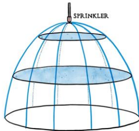
DISTRIBUTION PATTERN FROM A STANDARD SPRAY SPRINKLER
