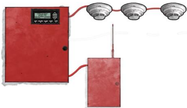
Household Fire Alarm System (Note the wiring and presence of a control unit)
